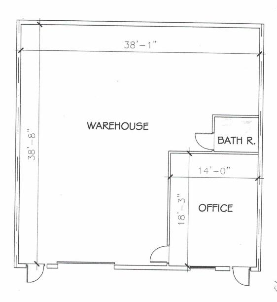
UNIT 6 FLOOR PLAN SCALE  $\frac{1}{8} = 1'$ - O"
