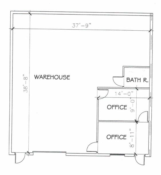
UNIT 8 FLOOR PLAN SCALE  $\frac{1}{8} = 1' - 0"$
