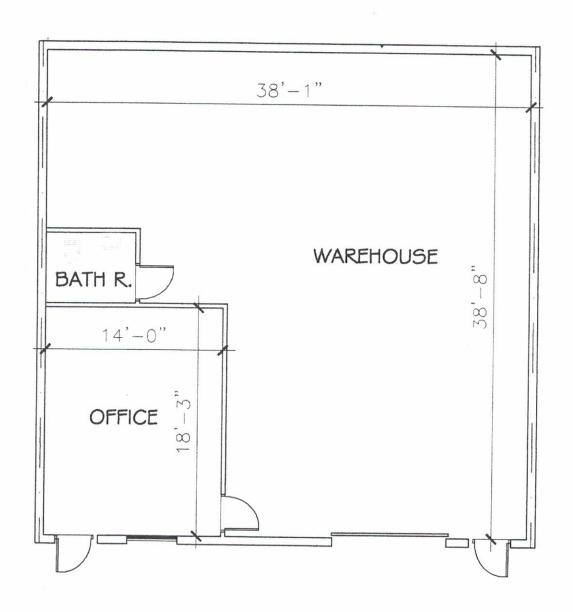
UNIT 5 FLOOR PLAN SCALE  $\frac{1}{8} = 1' - 0"$
